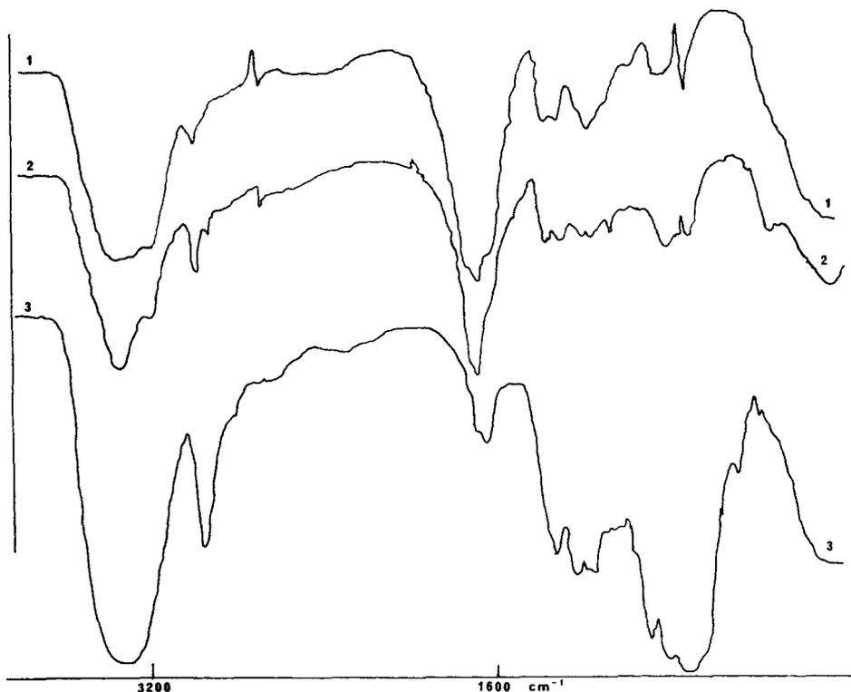
Fig. 1. IR spectra of (1) polyacrylamide, (2) PAM-*g*-cellulose (2:1), and (3)  $\alpha$ -cellulose.
